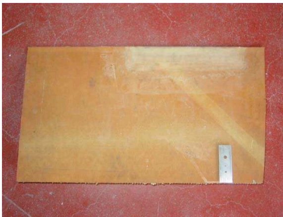
Figure 2 Left : composite part with hole type IQI,
